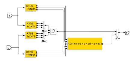
Error block for axis-angle representation of the orientation
