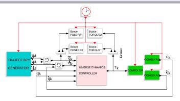
Block diagram for real time control with a set of COMEDI blocks
