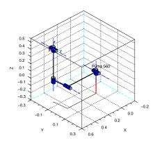
Standard DH-based Puma 560 at its zero angle pose
