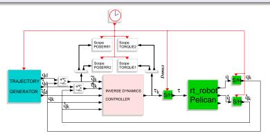
Scicos block diagram for the control system (real time control)
