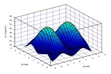
Inertia seen by the joint 1 of the r3 as a function of joint angles  $q_2$  and  $q_3$
