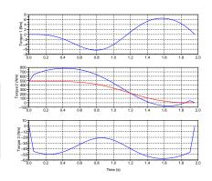
Joint torques for the given joint space trajectory (grav. torque in red)
