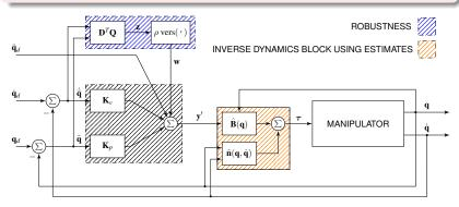
Block scheme of joint space robust control
