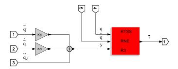
Inverse dynamics controller for the Manutec r3 robot
