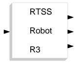
FDB ready to simulate the forward dynamics of the Manutec r3
