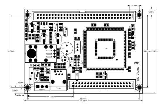
Figure 3.4: [FLEX001] Dimensions of FLEX Light Base Board
