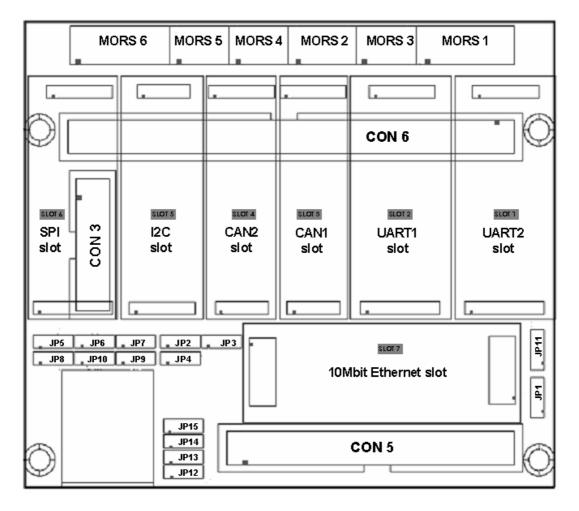
Figure 3.12: [FLEX101] Details of FLEX Multibus Base Daughter Board
