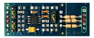
Figure 3.18: [FLEX104] FLEX Multibus RS485 Module
