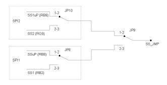
Figure 3.13: [FLEX101] SPI Chip Select (Slot6) Jumper Settings
