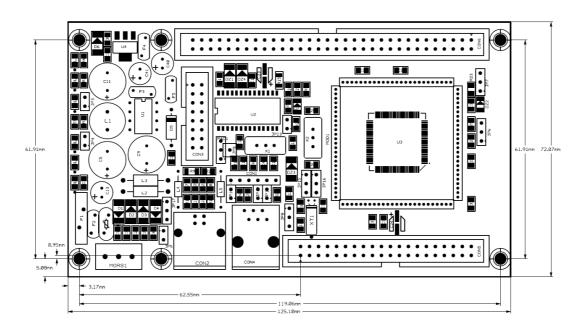
Figure 3.7: [FLEX003] Dimensions of FLEX Full Base Board
