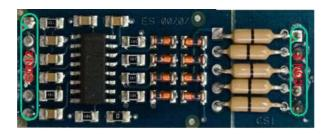
Figure 3.16: [FLEX103] FLEX Multibus RS232 Module
