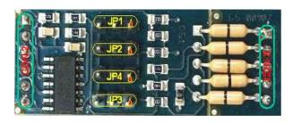
Figure 3.26: [FLEX108] FLEX Multibus Serial TTL Module
