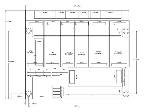
Figure 3.11: [FLEX101] Dimensions of FLEX Multibus Base Daughter Board
