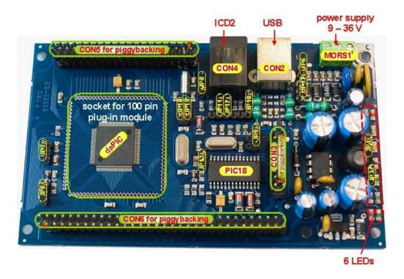
Figure 3.6: [FLEX003] FLEX Full Base Board
