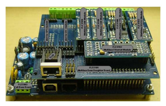
Figure 3.32: [FLEX110] FLEX multibus pack
