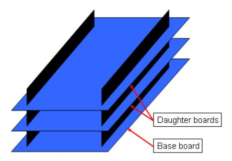
Figure 3.1: Piggybacking of FLEX Boards
