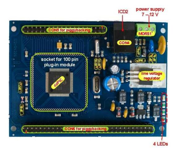
Figure 3.3: [FLEX001] FLEX Light Base Board
