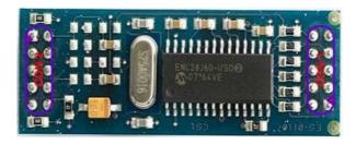
Figure 3.14: [FLEX102] FLEX Multibus Ethernet Module
