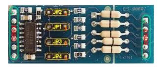
Figure 3.24: [FLEX107] FLEX Multibus SPI Module
