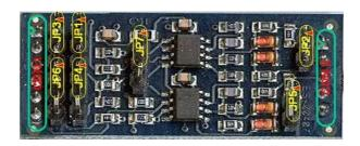
Figure 3.20: [FLEX105] FLEX Multibus RS422 Module
