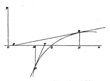
At the point R we have f(x) positive and f''(x) negative. Draw the tangent RS; then, starting from N the Newtonian approximation proceeds to S, and S and N are on *opposite* sides of Q. Moreover there is no security that QS is less than QN, and there is no security that the approximation can be continued from S. Thus the approximation cannot be safely begun from N.
