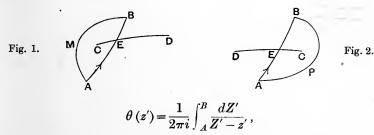
where the integration extends along an arc AB from A as the lower limit to B as the upper limit. When we take a closed contour of which AB is a portion, AB is the positive direction of description in figure 1 and is the negative direction of description in figure 2.
