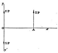
and  $\Sigma P$  acting along Oy' form this couple. The latter force is destroyed by the force  $\Sigma P$  along Oy. Hence the single resultant is  $\Sigma P$  acting at A, that is, at a point the distance of which from O is  $\frac{\Sigma Px}{\sum P}$ .
