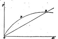
Here  $\phi(x) = 2\sqrt{(ax)}$ ,  $\psi(x) = kx$ , c = 0; h is to be found from the equation  $2\sqrt{(ah)} = kh$ ;
