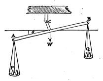
Let C be the fulcrum, h its distance from the straight line which joins A and B. Let W be the weight of the beam, k the distance of the centre of gravity of the beam from C; this centre of gravity being supposed to lie on the perpendicular from C on the straight line which joins A and B. Let S be the weight of each scale; so that P and S act vertically through A, and C and C vertically through C be the angle which the beam makes with the horizon when there is equilibrium.
