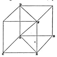
the resultant of this force and Z, that is, of the forces represented by AE, AD, is represented in magnitude and direction by AF, the diagonal of the parallelogram DE. Hence the resultant of X, Y, Z is represented in magnitude and direction by AF. Let R be the magnitude of the resultant, and a, b, c the angles the direction of R makes with those of X, Y, Z. Then, since
