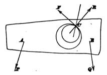
which passes a solid fixed cylindrical axis. Let the outer circle in the figure represent a section of the cylindrical hole made by a plane perpendicular to its axis, and the inner circle the corresponding section of the solid axis. In the plane of this section, we suppose two forces P and Q to act on the solid body at the points A and B. Also at the point of contact C there is a normal force R and a tangential force F. These four forces keep the body in equilibrium.
