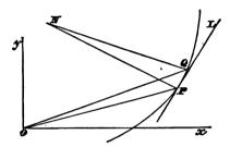
adjacent point; r,  $\theta$  the polar co-ordinates of P; let s be the length of the curve measured from some fixed point up to P, and  $PQ = \delta s$ . Draw PL the tangent at P; and PN, QN normals at P and Q respectively, then PN is ultimately the radius of curvature at P. Let T denote the tension at P,  $T + \delta T$  the tension at Q,  $Fm\delta s$  the force acting on the element PQ, which will ultimately be in the direction QP produced.
