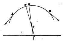
it leaves the curve. Let P,Q be adjacent points in the string; let the normals to the curve at P and Q meet at O; let  $\theta$  be the angle which PO makes with some fixed straight line, and  $\theta + \delta\theta$  the angle which QO makes with the same line. The element PQ is acted on by a tension at P along the tangent at P, a tension at P along the tangent at P, and the resistance of the smooth curve which will be ultimately along PO.
