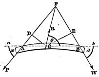
sure on the fulcrum, and  $\theta$  the angle which it makes with the straight line aCb; then if we apply a force R in the direction CR, we may suppose the fulcrum removed, and the body to be held in equilibrium by the forces P, W, R.
