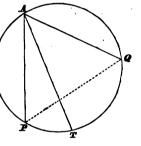
as the magnitudes of the forces are supposed unchanged, the magnitude of the resultant and the angles which it makes with the components remain unchanged. Hence if T be the intersection of the resultant and the circle originally, it will always be so, since the arcs PT and QT are proportional to the angles PAT and QAT; the resultant will therefore have turned through the angle  $\alpha$  round the point T.
