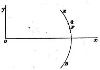
$$\bar{x} = \frac{a^2 \int_{-a}^{a} \cos \theta \, d\theta}{a \int_{-a}^{a} d\theta} = \frac{a \sin \alpha}{\alpha}.$$
