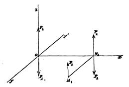
The moment of the first couple is  $P_1y_1$ , and this couple, without altering its effect, may be transferred to the plane of (y, z), which is parallel to its original plane. The moment of the second couple is  $P_1x_1$ , and the couple is in the plane of (x, z).
