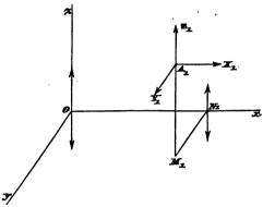
the direction of  $Z_1$  meet the plane of (x, y) at  $M_1$ , and draw  $M_1N_1$  perpendicular to Ox. Apply at  $N_1$  and also at O two forces each equal and parallel to  $Z_1$ , and in opposite directions. Hence  $Z_1$  at  $A_1$  or  $M_1$  is equivalent to  $Z_1$  at O, and two couples, the former having its moment  $= Z_1 \cdot N_1M_1$ , and which may be supposed to act in the plane of (y, z), and the latter having its moment  $= Z_1 \cdot ON_1$  and acting in the plane of (z, x).
