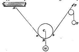
Let  $\alpha$  and  $\alpha'$  be the angles which  $A\alpha$  and Pb make with the vertical.
