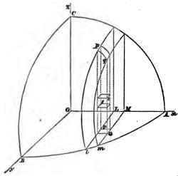
128. To find the centre of gravity of a solid we divide it into elements as follows: draw a series of planes perpen-
