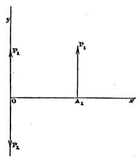
the plane of the forces as origin and draw rectangular axes Ox, Oy, the latter parallel to the forces. Let  $A_1$  be the point where Ox meets the direction of  $P_1$ , and let  $OA_1 = x_1$ .
