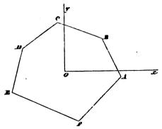
Let the sides of the figure ABCDEF represent the forces in magnitude and position; the first force being supposed to act in the straight line AB from A towards B, the second in the straight line BC from B towards C, and so on.
