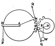
on the circumferences of which the teeth are arranged; C the point of contact of two teeth; QCQ a normal to the surfaces in contact at C. Suppose an axle is fixed on the wheel B, and the weight W suspended from it at E by a cord; also suppose the power P acts by an arm AD; draw Aa, Bb perpendicular to QCQ. Let the mutual pressure at C be Q. Then, since the wheel A is in equilibrium about the fixed axis A, the sum of the moments about A equals zero; therefore
