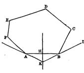
rods as AB. This rod is acted on by a force at the middle point H at right angles to AB, and by actions from the hinges at A and B. The former force is proportional to AB, and may be denoted by  $\mu .AB$ . The three forces must meet at a point, suppose K; then by resolving parallel to AB, we find that the actions at A and Bmust be equal; we will denote
