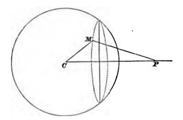
attracted particle. Let CM=r, PM=y, CP=c,  $\theta=$  the angle PCM,  $\phi=$  the angle which the plane PCM makes with the plane of the paper,  $\delta r=$  the thickness of the shell, and let  $\rho$  denote the density of the shell.
