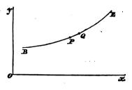
Let P, Q, be adjacent points in the exterior generating curve; suppose B a fixed point in the curve, let BP = s, and  $PQ = \Delta s$ ; let x, y be the co-ordinates of P; k the thickness of the shell at P. The volume of the element contained between two planes perpendicular to the axis of x through P and Q respectively is ultimately  $2\pi yk\Delta s$ , and the abscissa of the centre of gravity of this element is ultimately x; hence
