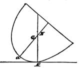
the axis of the parabola further from a than G is, and the equilibrium is *stable*.
