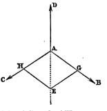
the resultant of the two forces which AG and AH respectively represent.
